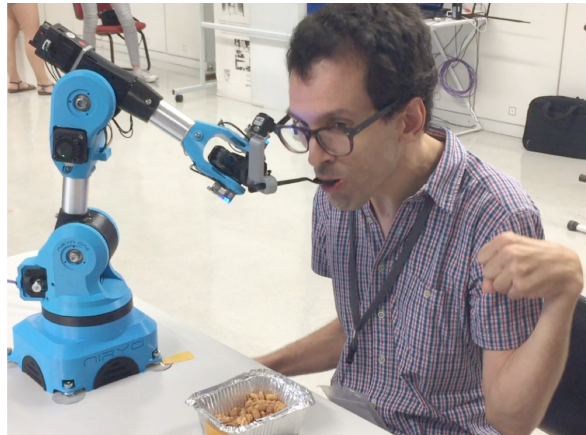
Figure 3.1: Our Niryo One assistive-feeding robot
