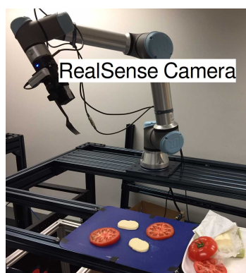
(a) UR5 with wrist-mounted camera (b) Wrist camera view with identified food
