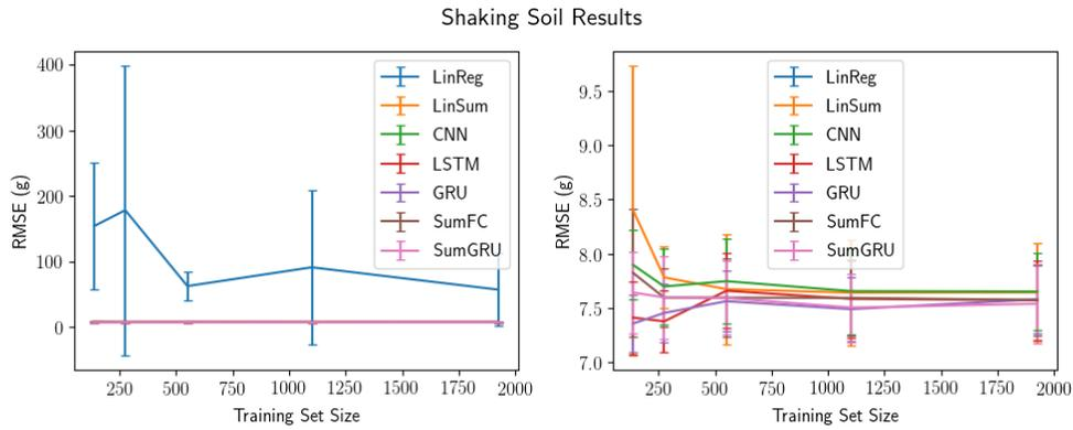
Figure 24: Training curves showing variation in performance of models with different sized training sets of *shaking soil data*. Results are from averaging over 5 trials. **(Left)** Results from all models. **(Right)** Results from regularized linear regression omitted to show detail of other models' performances.
