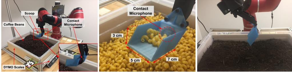
Figure 1: **(Left)** The robotic granular material manipulation setup used to collect a dataset. **(Center)** The scoop in its *resting position*, prepared to pour or shake cellentani pasta. The silhouette of the contact microphone is visible through the back of the translucent basin of the scoop. **(Right)** The robot with its scoop at its maximum pouring angle, a 60 degree pitch, with the peat top soil below its scoop.
