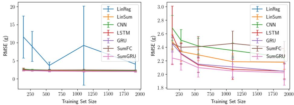
Figure 29: Training curves showing variation in performance of models with different sized training sets of *pouring coffee* data. Results are from averaging over 5 trials. **(Left)** Results from all models. **(Right)** Results from regularized linear regression omitted to show detail of other models' performances.
