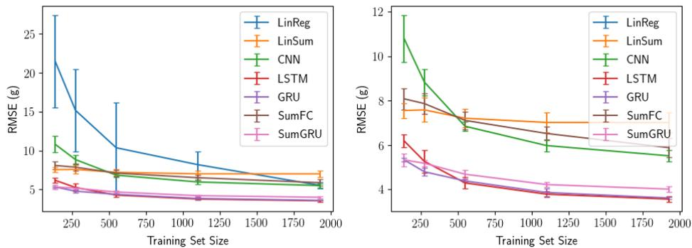
Figure 30: Training curves showing variation in performance of models with different sized training sets of *shaking coffee* data. Results are from averaging over 5 trials. **(Left)** Results from all models. **(Right)** Results from regularized linear regression omitted to show detail of other models' performances.
