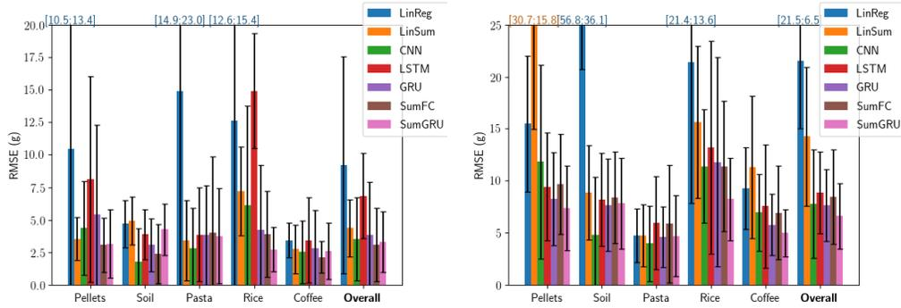
Figure 18: Performance of single-material models on estimating mass during leave-one-level-out cross-validation. Bars that surpass the bounds of the graph have their inter-trial means and standard deviations respectively printed above them. **(Left)** Estimating poured mass. **(Right)** Estimating shaken mass.
