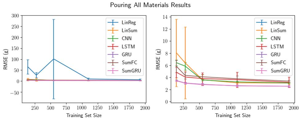
Figure 19: Training curves showing variation in performance of models with different sized training sets averaged over data from pouring all materials. Results are from averaging over 5 trials. **(Left)** Results from all models. **(Right)** Results from regularized linear regression omitted to show detail of other models’ performances.
