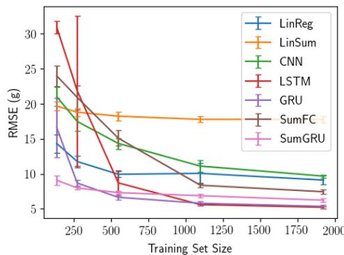
Figure 22: Training curves showing variation in performance of models with different sized training sets of shaking pellets data. Results are from averaging over 5 trials.
