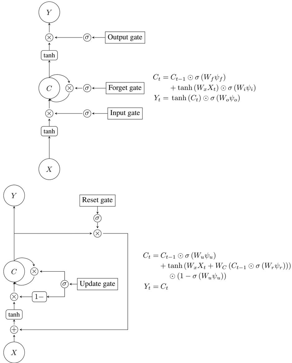
Figure 15: Comparison of **(Top)** LSTM and **(Bottom)** GRU memory cells. For both diagrams,  $X$  is the input,  $Y$  is the output, and  $C$  is the memory vector.  $W$  refers to a learned matrix.  $\psi$  refers to an input vector composed by concatenating  $X$  and  $Y_{t-1}$ .  $\odot$  is the Hadamard product.  $\sigma$  is a sigmoid with range  $[0, 1]$ .
