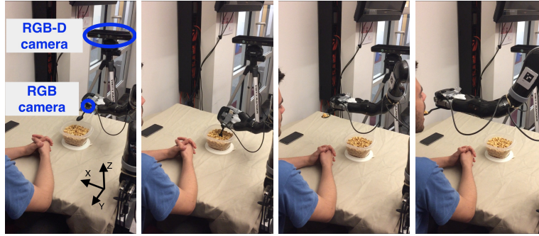
Fig. 1: Our feeding system includes a MICO robot arm, an RGB-D camera, and an RGB camera. The first image also labels the axis orientations of the robot coordinate system.
